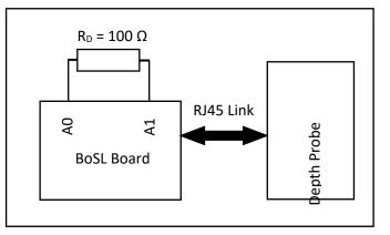
In this design a MS-5803 located on the BoSL board is used to capture the current air pressure so water depth can be calculated via:  $D = (P_{probe} - P_{air})/(\rho_{water}g)$ . A voltage divider is used to measure the resistance between the EC pins.  $R_D$  is chosen to be 100  $\Omega$  for this as it makes the range of EC values commonly expected in water systems to be easily readable. The resistance between the EC pins is given by  $R_{EC} = R_D (V_{ECD}/V_{CC} - 1)$ .
