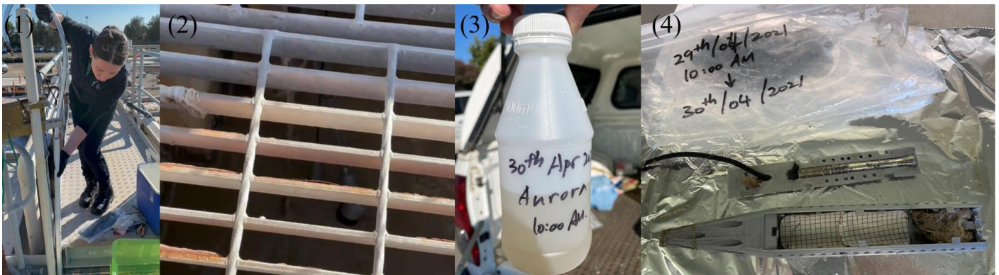
Figure 5. Trial Deployment. (1) Both MAD-AS and the passive sampler were deployed at the same location at the treatment plant inlet. (2) Samplers submerging in the wastewater flow. (3) Sample collected by MAD-AS. (4) The passive sample under pre-processing in the laboratory.
